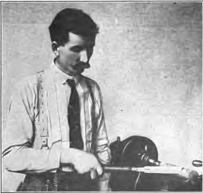
Fig. 26. Turning with One Hand.
